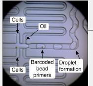
Microfluidic device sorts and process cells
